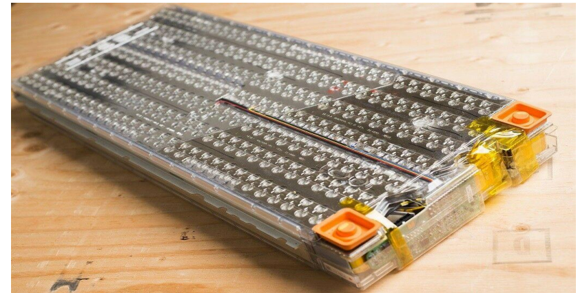
Tesla Model S/X Battery Module (74P6S)
