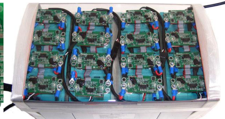
48V 20Ah battery with 16 pcs BMS Slave Module
