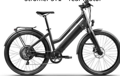
Stromer ST1 – rear motor
